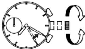
It is recommended that the hands be set to the time a few minutes ahead of the current time, taking into consideration the time required to adjust the stopwatch hand position if necessary.
